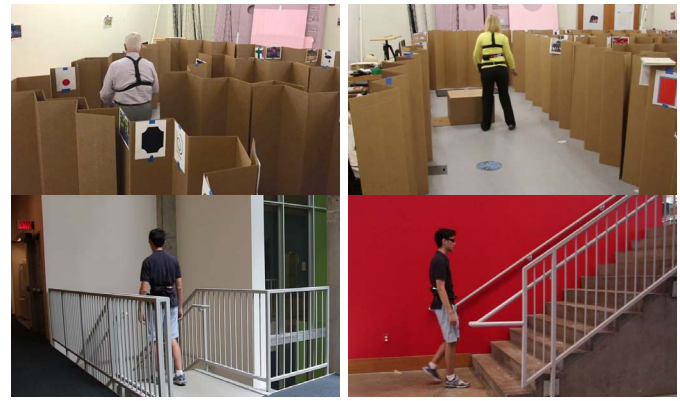
Fig. 7. Experimental Setups: Top left shows the subject wearing ALVU within a hallway test scenario. Top right shows a low obstacle avoidance scenario; the subject is stepping to the right to pass the box. Bottom left shows a staircase down test. Bottom right shows a staircase up test.
